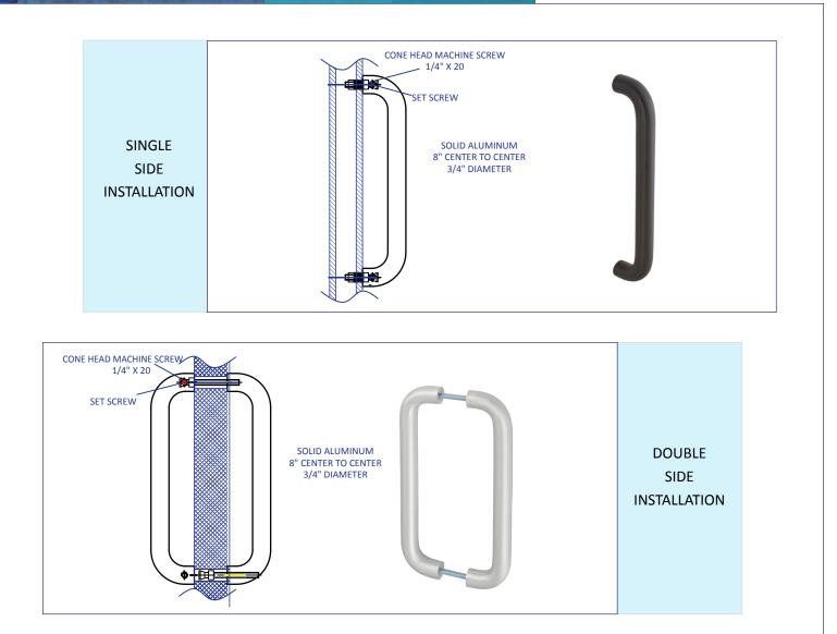
Rockwell Solid Aluminum Inline handles are available in single side or back to back handles.
