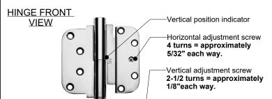
Hinges are preset in the mid-position. to allow a 4 way adjustment
