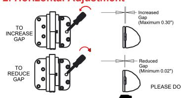
Adjust hinges as needed. Only 4 turns max are needed each way to either close or increase the gap
