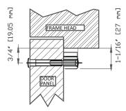
4. WITH THE TRACK INSTALLED ON THE DOOR AT DIMENSION "A", LOCATE DIMENSION "C" AND DRILL A 5/16' DIAMETER HOLE AND INSTALL SEX BOLT "A" AND SECURE WITH SCREW B TO COMPLETE INSTALLATION.
