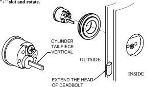
5. From the inside of the door orient the turn piece mounting plate and secure by inserting the two 2" pan head machine screws through the turn piece mounting plate, lock, and into the cylinder housing.
