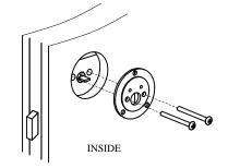
6. Install the turn piece trim by positioning the turn piece over the mounting plate, inserting the cylinder tailpiece into the turn piece. Secure the turn piece in place by fastening two 1/2" turn piece mounting screws through the two countersunk holes on the turn piece.
