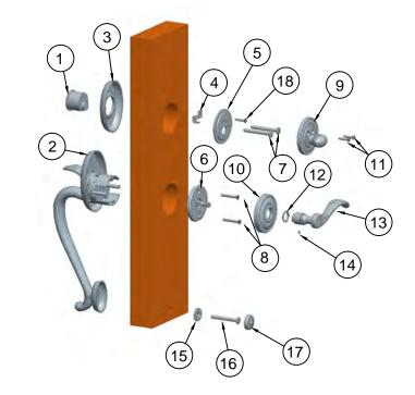
A. Using the marking template for handleset, mark hole E and drill 3/8" hole as specified.
