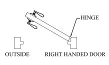
2. The handle set is preset to work with a left hand door, should you have a right hand door, the left handed spindle cartridge will need to be switched to a right hand spindle cartridge.
