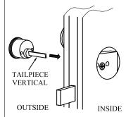
10. From the inside of the door, orient the deadbolt mounting plate and secure by inserting the two deadbolt mounting screws through the deadbolt mounting plate, lock, and into the cylinder housing.
