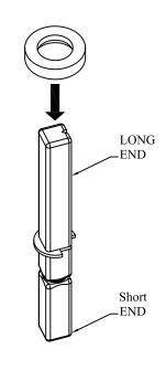
5. From the inside of the door insert the short end of the spindle into the latch of the lock ensuring the groove side of the long end of the spindle is facing down.
