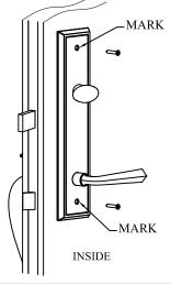
15. Align the external pull MARK assembly with the edge of the door and mark the position of the top and bottom screw hole locations. Drill a  $\frac{1}{8}$ " pilot holes and secure the external pull assembly in MARK place with three wood screws. OUTSIDE
