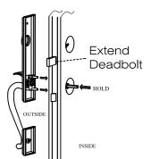
7. Hold the external pull assembly in place the latch mounting plate onto the spindle. Secure the latch mounting plate using the two latch mounting plate screws.
