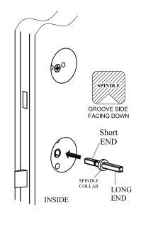
6. Holding the spindle in place from the inside of the door, slide the spindle and from the inside of the door slide cartridge of the external pull assembly onto the spindle. Holding spindle, test thumbpiece to retract latch.
