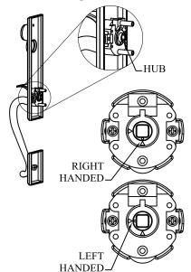
3. For a right hand door, please replace the spindle cartridge with the correct right hand spindle cartridge. Right hand spindle cartridge (included) has instructions on changing the cartridge from left hand to right hand.
