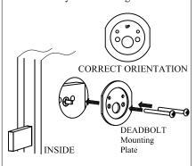
11. Position the internal plate assembly over the mounting plate and insert the cylinder tailpiece into the thumbturn of the internal plate assembly.
