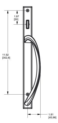
Mounting screws: 2 Phillips Oval Head machine screws.
