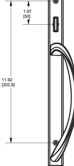
Mounting screws: 2 Phillips Oval Head machine screws.
