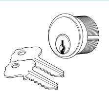
Mortise Cylinder Specifications Construction: Zinc diecast housing Mortise Shell cover - Aluminum Anodized Cover Keys: Solid Brass Nickel Plated Keys Trim Ring: Extruded or Stamped Aluminum Thumbturn: Zinc diecast 5 pin cylinder with SC1 keyway, pin depths and increments. Cylinder length: 1"
